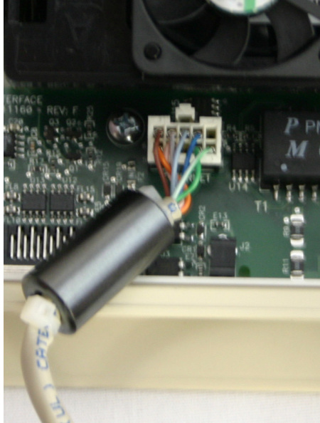
FIGURE 8-15: ETHERNET TO SYSTEM BOARD CABLE CONNECTION
