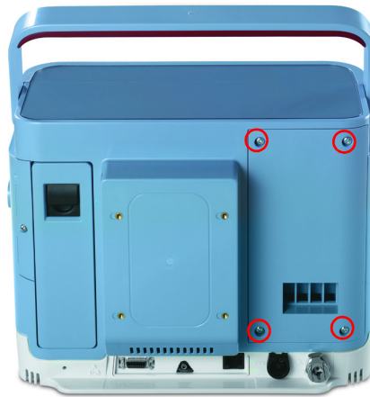
FIGURE 8-2: AIR PATH ASSEMBLY SCREW LOCATIONS
