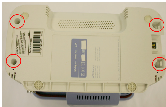
FIGURE 8-6: BOTTOM ENCLOSURE SCREW LOCATIONS
