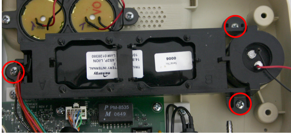
FIGURE 8-13: CAPACITOR/INTERNAL BATTERY FAN RETAINER SCREWS
