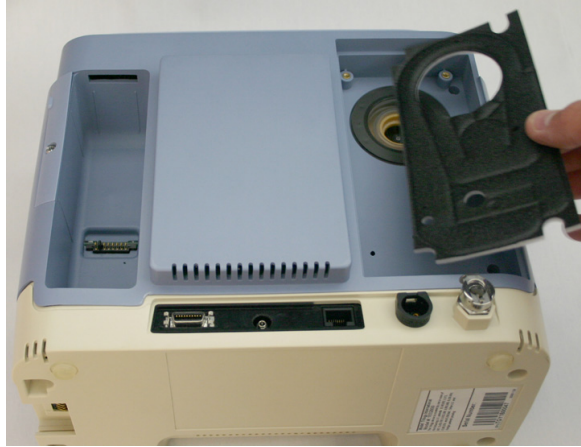
FIGURE 8-4: AIR PATH FOAM REMOVAL/INSTALLATION
